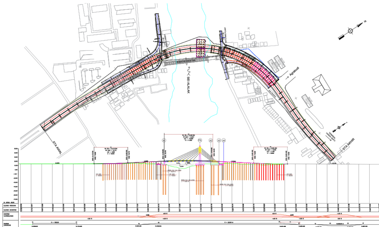
Fig 1. Plan layout of Sei Alalak Bridge
