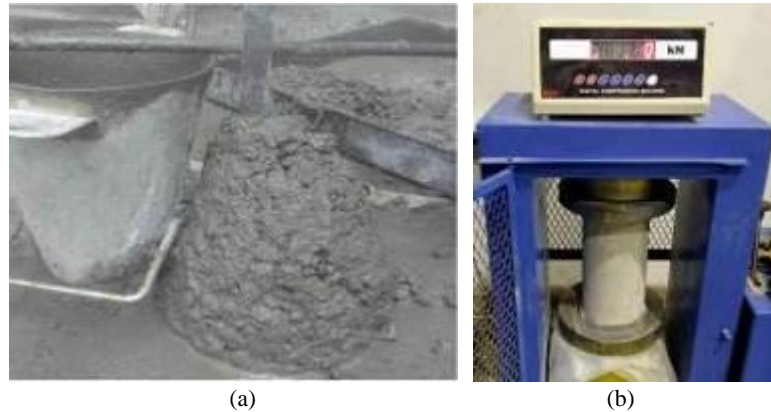
Fig 4. Testing programs on fresh and hardened concrete: (a) slump test to determine the workability of fresh concrete; (b) compressive strength test setup
