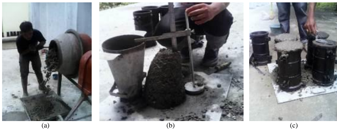
Fig 2. Concrete sample preparation. (a) concrete mixing process, (b) slump measurement to determine consistency, (c) Pouring concrete into cylinder molds
