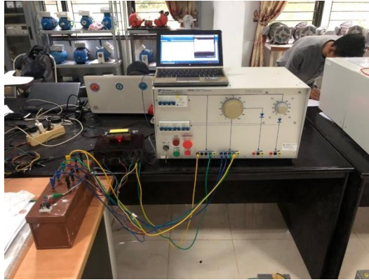
Fig 3. PZEM-004t sensor voltage test
