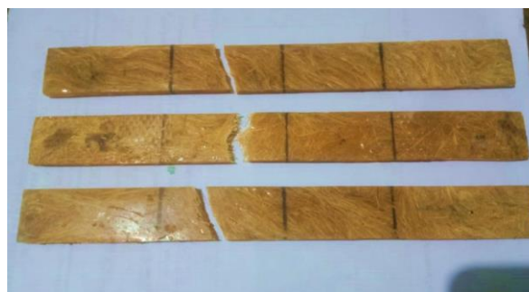
Fig 17. Tensile Test Results of Gigantochloa Apus
