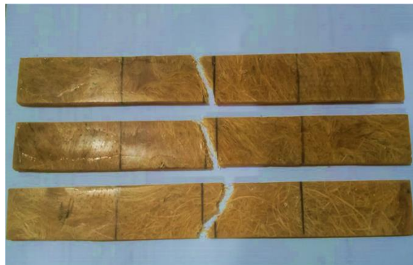
Fig 15. Tensile Test Results of Bamboosa Blumeana
