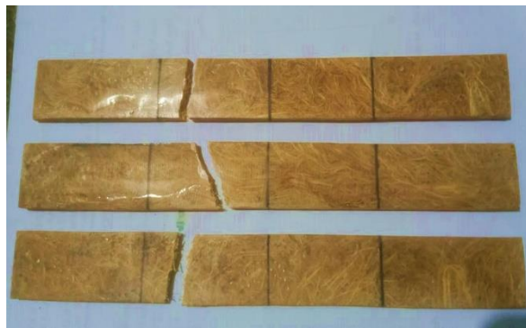
Fig 16. Tensile Test Results of Bamboosa Vulgaris
