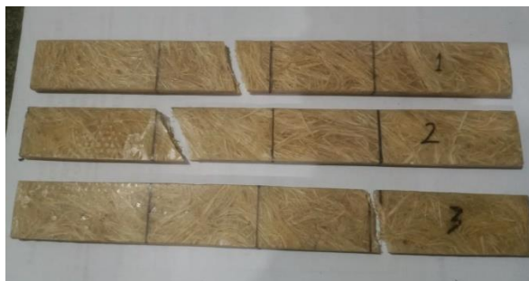
Fig 18. Tensile Test Results of Gigantochloa Apus no-treatment
