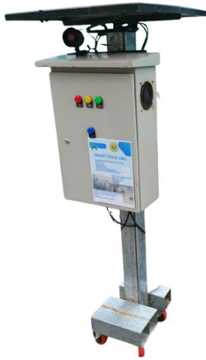
Fig 2. UNJ Smart Stick, the device to measure flood and environmental parameters
