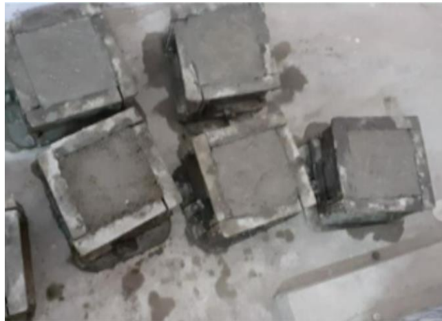
Fig 2. Concrete Specimens in Molds after Casting, Beginning the Curing Process to Achieve Required Strength.
