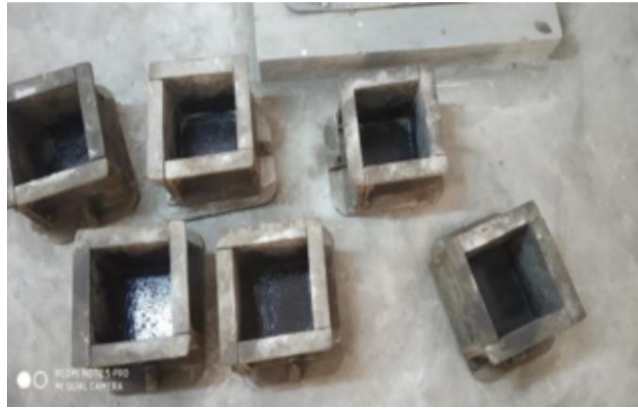
Fig 1. Concrete Molds Prepared for Casting Rebar Sleeve Grouting Specimens, Showcasing the Setup Prior to Concrete Pouring.
