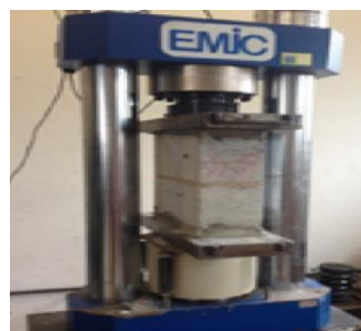
Fig 3. Reference Destructive Test Experimental Setup
