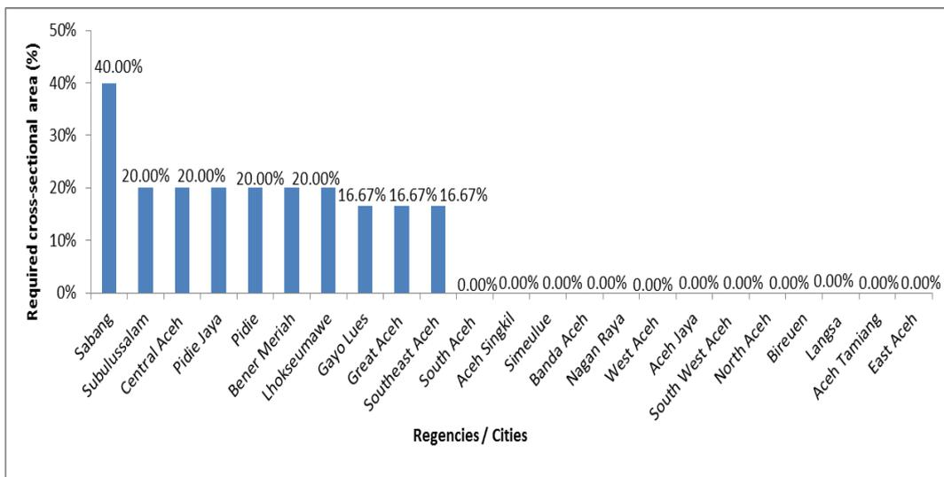
Fig 4: Comparison of the required cross-sectional area of the beam based on SNI 03-1726-2012 and SNI 03-1726-2019
