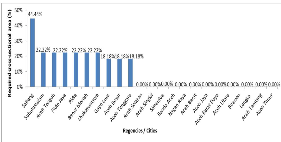
Fig 5: Comparison of the required cross-sectional area of tie beams based on SNI 03-1726-2012 and SNI 03-1726-2019
